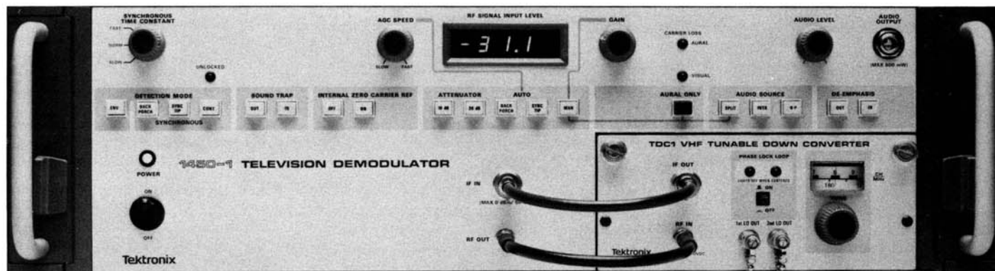
The 1450-1 is compatible with System M Television Transmission, the 1450-2 is compatible with System B/G, and the 1450-3 is compatible with System I.
